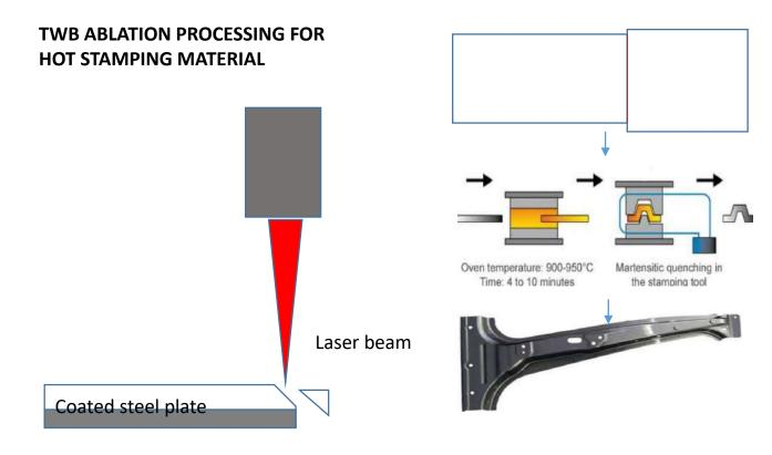
Hot stamping part have light weight with high strengths of 1,500 Mpa. But because of high strengths, stamping part cannot absorb impact. Hence, in somewhere of stamping part, less strengths part material is required. For this purpose, Tailor welded blank is required to weld different material has different physical properties.
